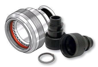
Constant Force Spring adaptors feature a fatigue and corrosion resistant steel band to terminate the cable screen. The resulting 360° termination creates an effective electrical connection, providing screen continuity between braid and adaptor.
